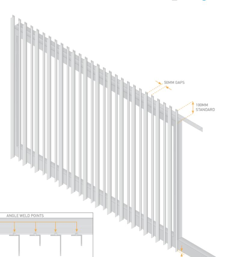
TOP ELEVATION DETAIL OF 50 X 25MM; 25 X 25MM STYLE
